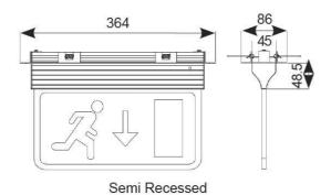
**ACCESSORIES** AE3LED/L/AD EAGLE LED DOUBLE SIDED LEGEND - ARROW DOWN AE3LED/L/AU EAGLE LED DOUBLE SIDED LEGEND - ARROW UP AE3LED/CPA/SI Eagle 3-in-1 Exit Sign Ceiling Plate Accessory AE3LED/SWB/SI Eagle 3-in-1 Exit Sign Side Wall Bracket Accessory
