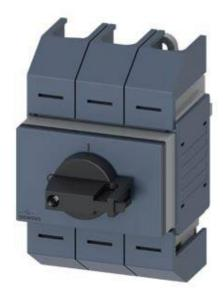
Switch disconnector 125A, size 02, 3-pole Front operating mechanism center Complete unit with direct operating mechanism gray Box terminal
