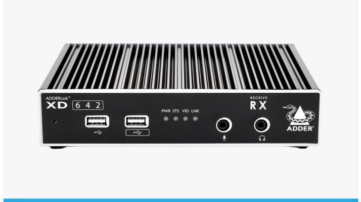
**A high-resolution, dual-head KVM extender with DisplayPort connectivity. Ultra-high definition 4K60 video, USB2.0 and audio are transmitted on a single CATx or fiber cable.**
