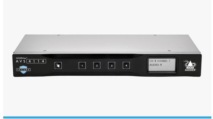
**Secure KVM switch for sharing single-head 4K video, USB keyboard and mouse, plus analog audio between four computers spanning multiple security classification levels.**
