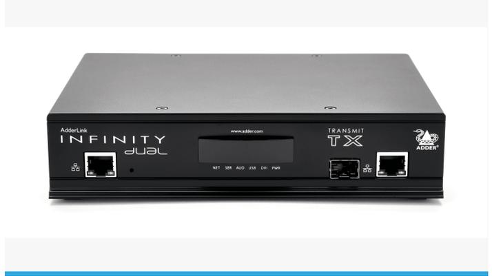
**A dual-link, dual-head digital video and USB fanless KVM extender that runs over a single cable on your standard IP network. Available with fiber access modules.**
