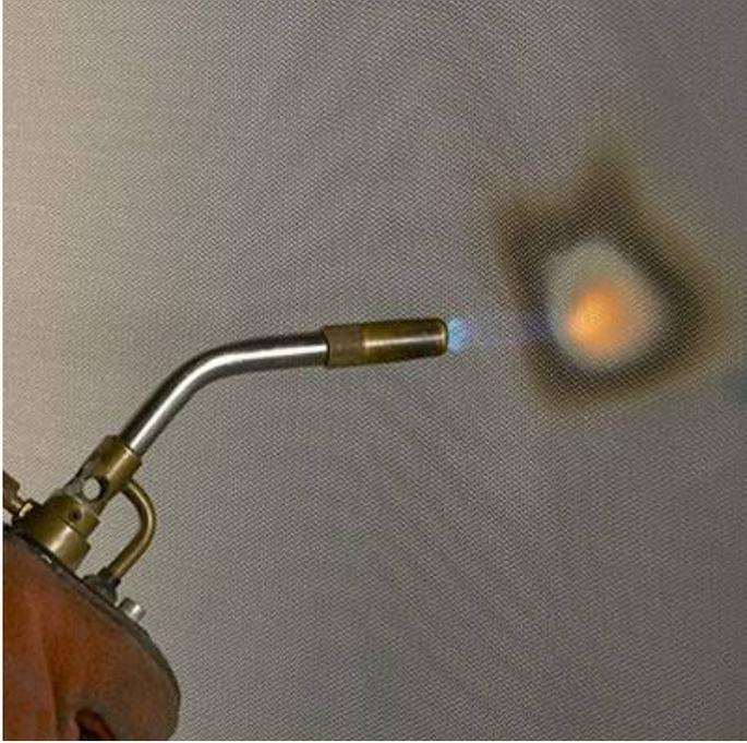
Firescreen is manufactured with non-flammable woven glass fibre and coated on both sides with a specially formulated micronized aluminum polymer, this Flame Retardant Firescreen is ideal for situations where fire integrity is crucial.
