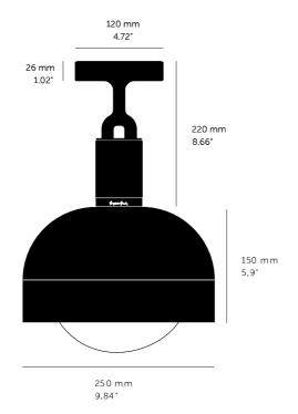
Ceiling light 1x solid metal lamp holder E27 / 220-240 VAC / IP20 Max 7.5W Bulb included CB Certified / Class 1 250 mm 1x solid metal light shade 1x hand-blown glass globe
