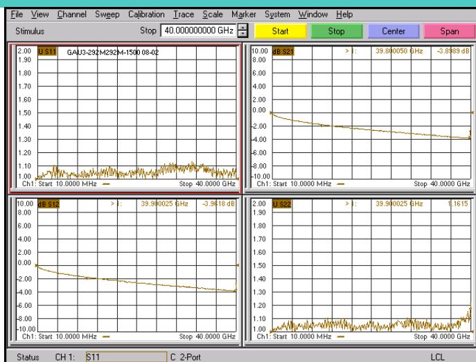
\*Note: Test Cable Assembly Length = 1500 mm
