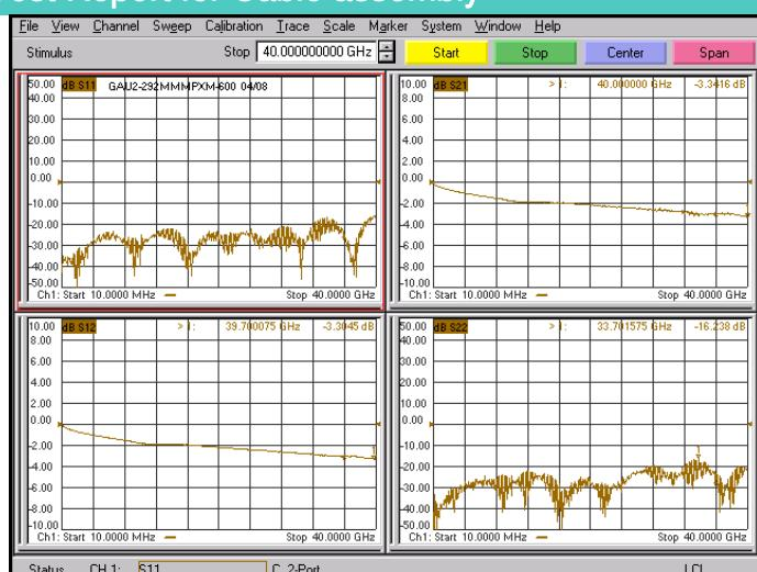
\*Note: Test Cable Assembly Length = 600 mm
