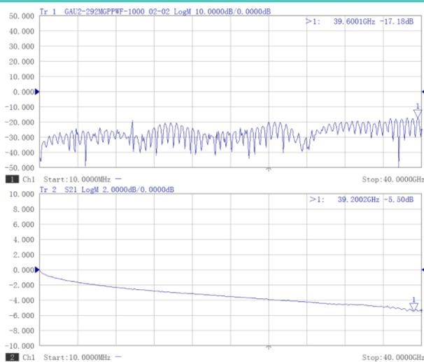
\*Note: Test Cable Assembly Length = 1000 mm
