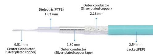
**P/N: FRF71-24FGPF-XXX****2.4mm Female to GPO(SMP) Female Cable Assembly | RG-405SS Flexible Coax Cable | DC - 50GHz****Electrical Data****Electrical Specifications for Different Length**
