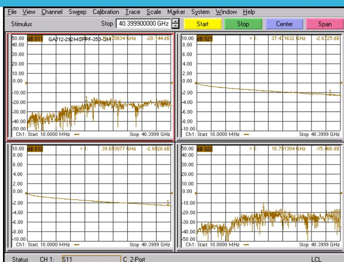
\*Note: Test Cable Assembly Length = 350 mm
