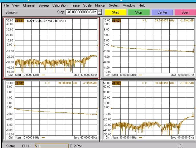
\*Note: Test Cable Assembly Length = 280 mm
