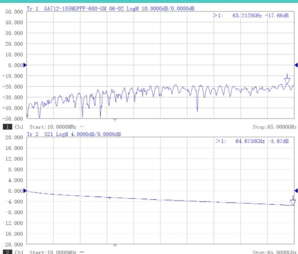
*\*Note: Test Cable Assembly Length = 600 mm*
