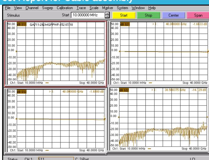
\*Note: Test Cable Assembly Length = 152 mm
