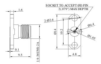
For Glass-bead of 0.51mm Pin Diameter
