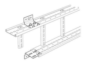
Wall support brackets are an effective way of fixing any width of ladder, running either vertically or horizontally, to a vertical support. These brackets can be mounted onto Swiftrack channel, structural steelwork or directly to a wall using M10 bolts (n
