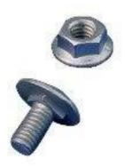
Compared with conventional nuts and bolts, quick bolt fasteners are a stronger, faster, easier and safer method of joining together tray. Square-shafted quick bolts lock firmly into position before fixing. The nuts, which have integral washers and a serra
